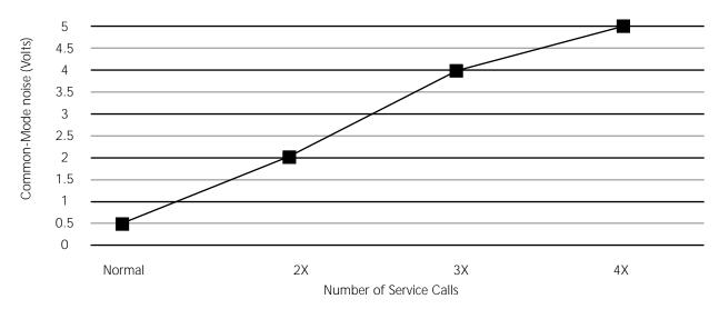
Fig 10: Imaging System Trial #5: The relationship between common-mode noise and service calls
