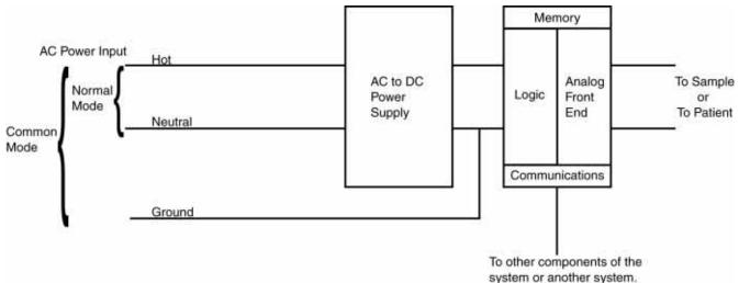
Fig 5: Medical System Block Diagram
